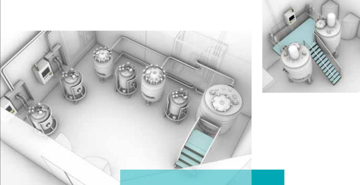
Concept study for planning of a LVP system with stationery and mobile process vessels
