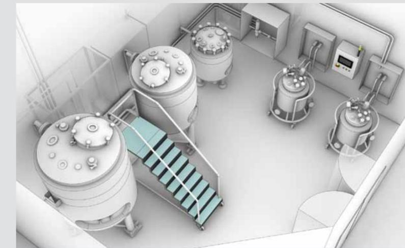
Factory layout with several formulation systems for different batch volumes with stationery and mobile process vessels
