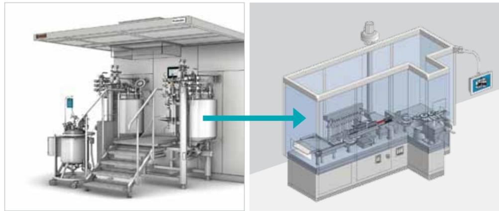
Pre-configured line concepts allow the safe and loss-free transfer of liquid products from the formulation system to the filling machine
